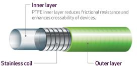
Catheter reinforced by stainless steel coil maintains the lumen even in flexural area.
