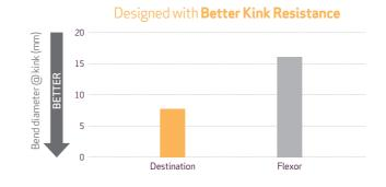
**Test Protocol** This test measured the bend diameter just before the sheath kinked.
